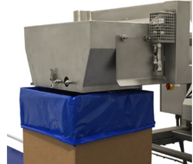
Filling straight into the box
