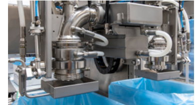
90° curved valve with drip catcher
