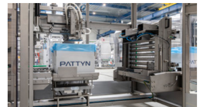
Tilttable infeed conveyor for easy cleaning
