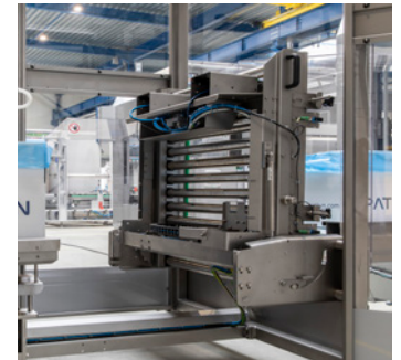
Tiltable infeed conveyor for easy cleaning
